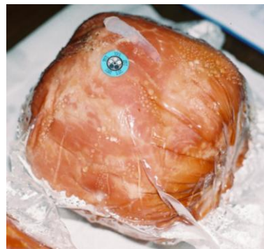
Figure 2. Self-adhesive temperature indicator, placed on the surface of packaged products.
